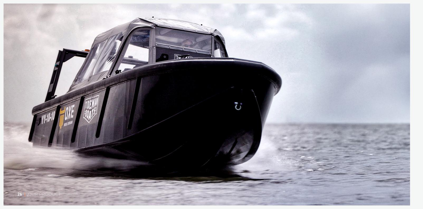
**SHELTAIR® X TIDEMAN** - This SHELTAIR® is designed for maximum protection and high speed usability. This model covers the entire sitting area (including captain). Cover is removeble in sections, creating different use scenarios. With this SHELTAIR®, TIDEMAN was able to hit a speed of 50 knots without any stress on the SHELTAIR®.
